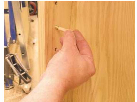
▲ Pic.17 Glue the shelf support sockets into their holes with epoxy adhesive. Push them in using a piece of dowel
